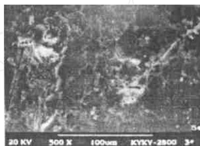
(a) Plastic deformation and spall
