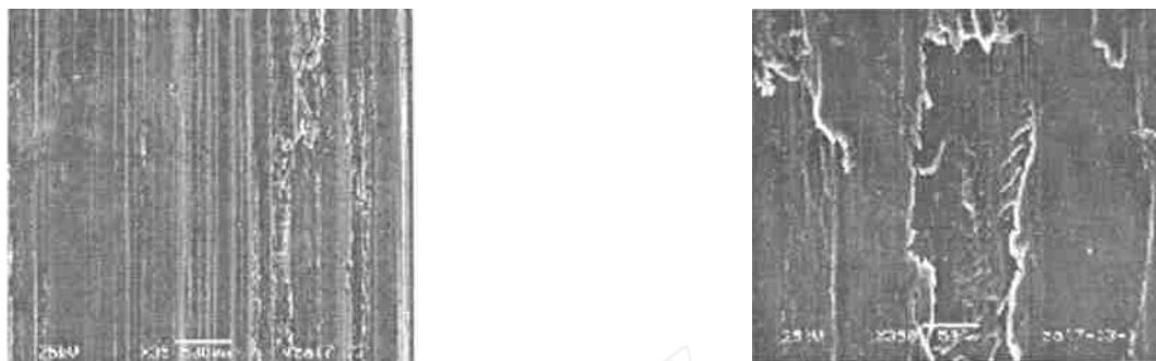
(a) Low magnification SEM picture of the 2024 aluminum alloy worn surface (35 ×)
