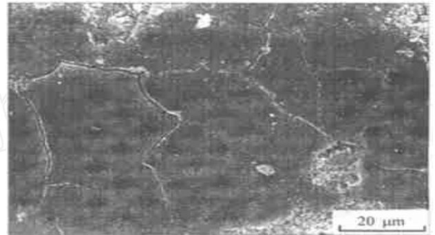
Fig 6 SEM photograph of the network cracking for Cr 2 O 3 coating
