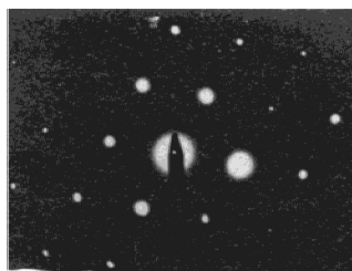
Fig. 8 Electron diffraction pattern of 316SS after Al implantation
