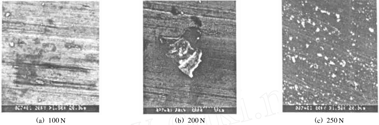
Fig 3 SEM morphologies of worn surfaces of EAMC at low, medium, and high load
