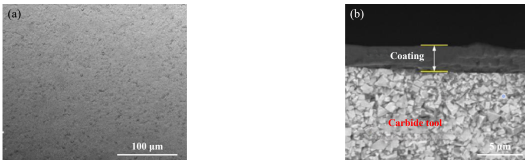
Fig. 6 SEM micrographs of (a) surface micro-morphology and (b) cross-section micro-morphology of coated tool [61]
