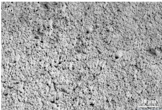
Fig. 17 SEM micrographs of micro morphology of crack propagation region of fatigue fractograph:
