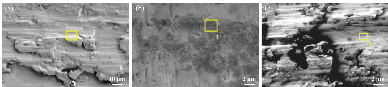
Fig. 6 SEM micrographs of worn surface on substrate TC4: (a) 35 °C-0W-20, (b) 35 °C-SPF Mo, (c) 90 °C-SPF Mo
