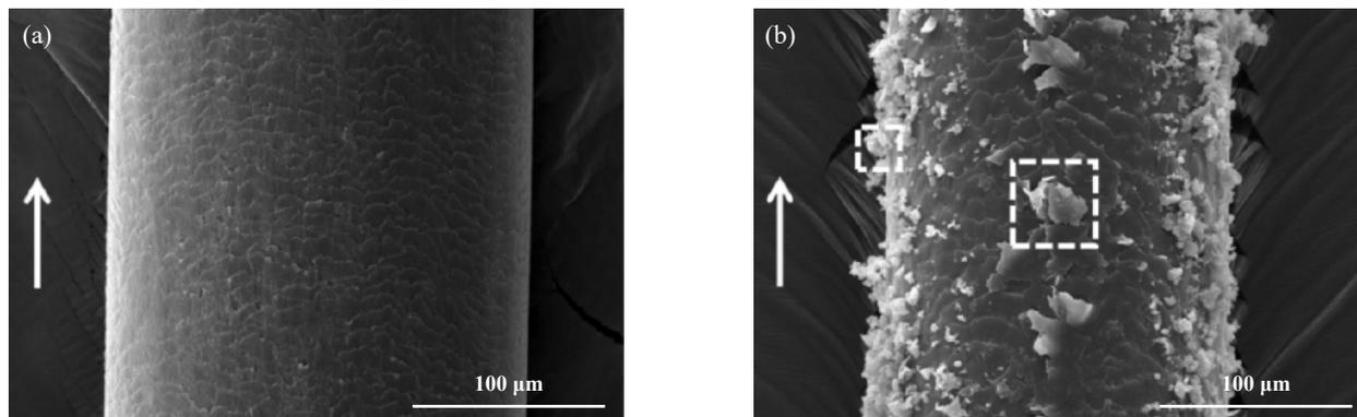
Fig. 2 FESEM micrographs of (a) horsehair without rosin (arrow indicates nap down), (b) horsehair with burnished rosin
