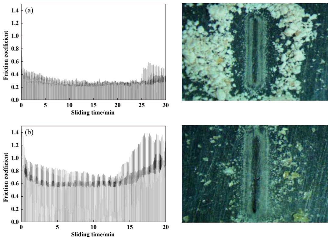
Fig. 3 Frictional traces and OM micrographs worn surfaces using (a) fine rosin powder and (b) coarse rosin powder. The rosin powder is prepared using Pirastro 9012 for cello.
