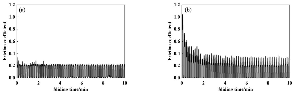
Fig. 4 Frictional traces of rosin coating by (a) solvent-evaporation and (b) melting-solidification in sliding against a GCr15 ball
