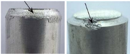
(a) Wear on the end of the bar (b) Damage on the V-shaped groove
