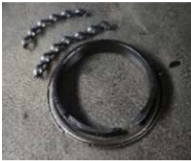
(c) Damaged bearing
