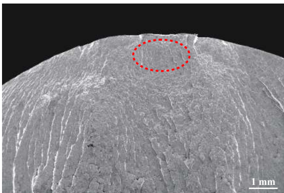
(a) Bending fretting fatigue fracture
