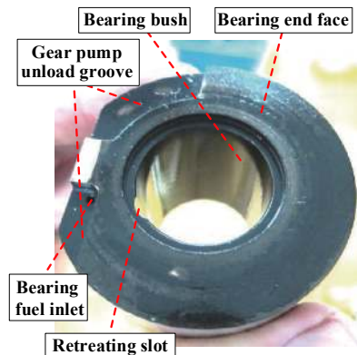
Fig. 1 Sliding bearing of aviation fuel gear pump 图1 航空燃油齿轮泵滑动轴承
