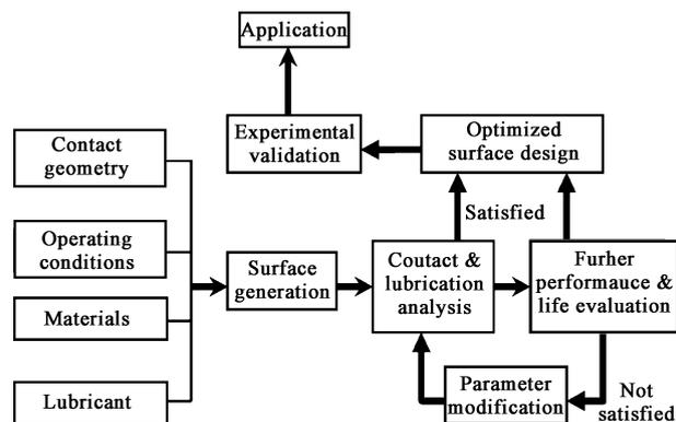
Fig. 2 Logic of the virtual surface texturing technology<sup>[32]</sup>
