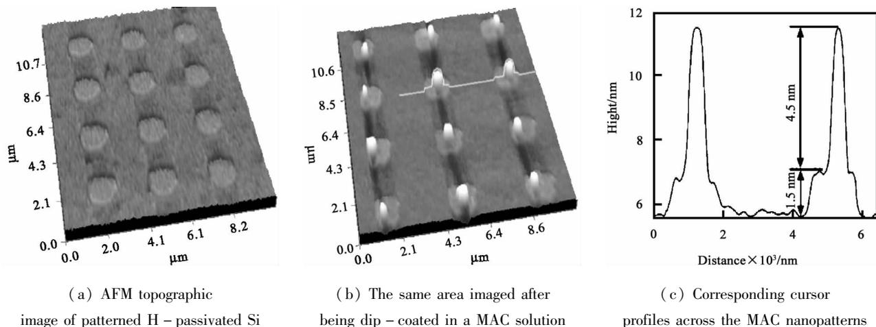
Fig. 3 Formation of nanopatterns and MAC lubricant layer<sup>[49]</sup>
